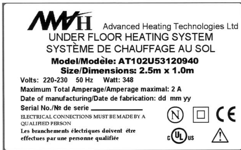
Figure 3 – Etiquetage des "Trame Chauffante AHT"
